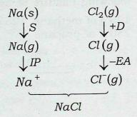
So,  $-Q = S + IP + \frac{1}{2}D - EA - U$ , where S is the heat of sublimation, IP is the ionization potential of Na, D is the dissociation energy, EA is the electron affinity, U is the lattice energy and Q is the heat of formation. On rearranging it
